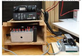
←The FT817 sitting on top of the LDG ProII tuner and underneath that is my CMOS III keyer with Galbraith paddle on RHS.
