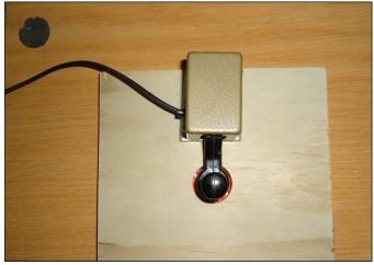
Mounted USSR key with cut-out to allow contacts to close properly.
