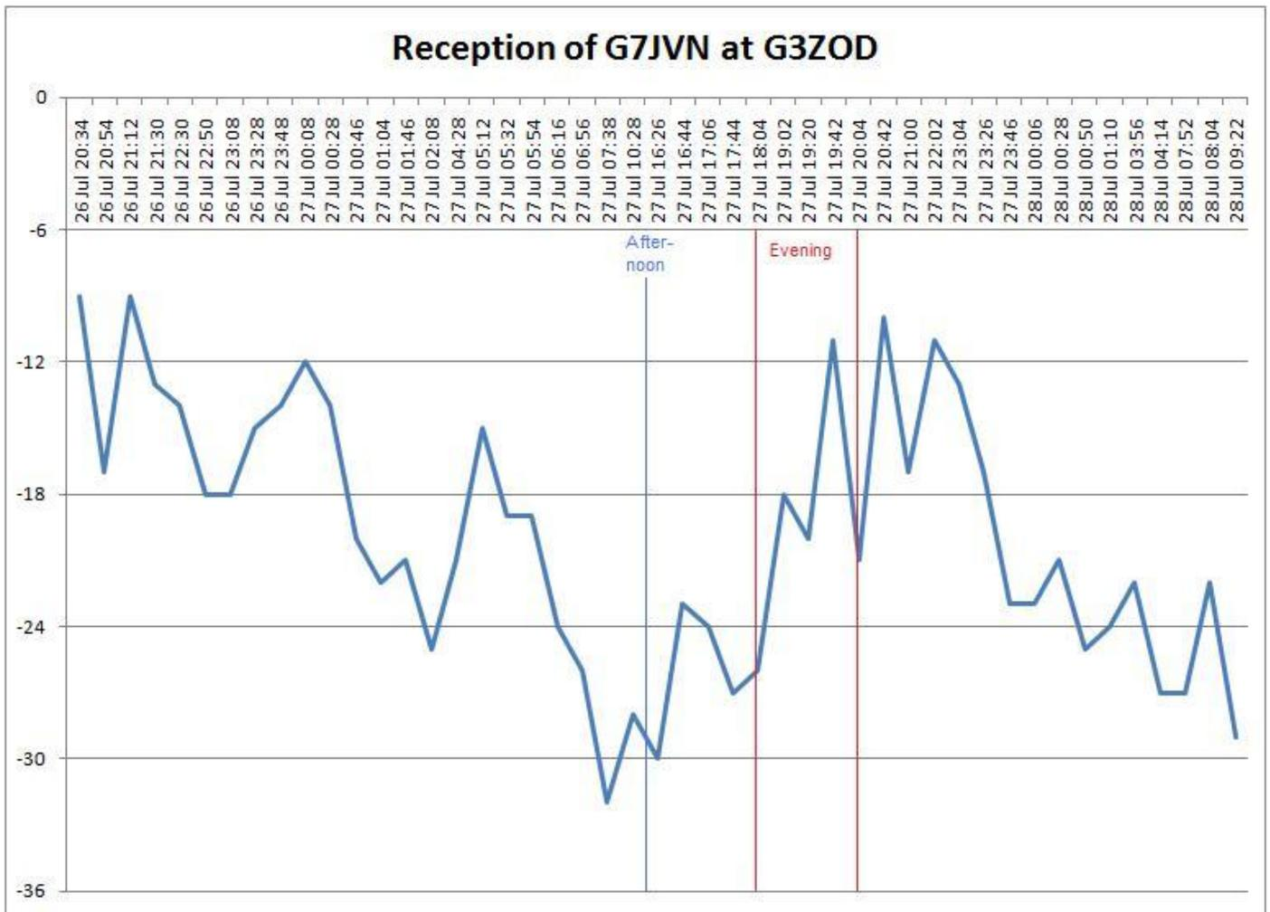
The vertical axis shows the signal strength in dB, so the higher the line, the stronger the signal.
