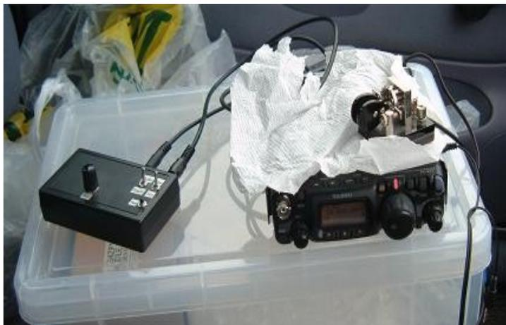
The second photo shows the station in the car, with my PK4 keyer, FT-817 and the G4ZPY miniature paddles with magnetic base. The paper is so I can rest my hand on the FT-817 without messing up the paint work!
