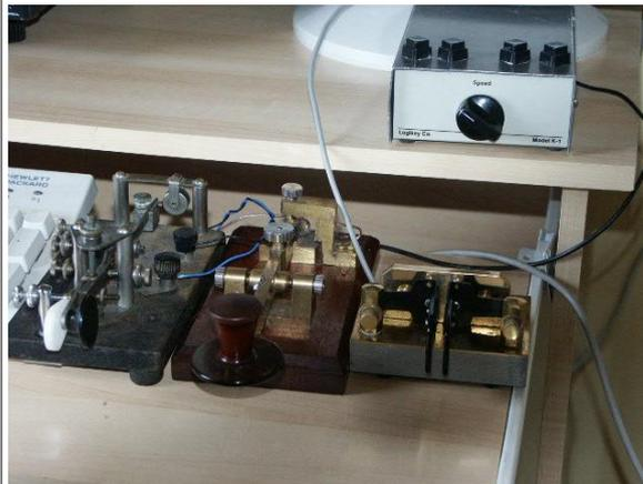
Hi Robert, as promised, a photo of me with the station used in SKW, the key is a copy of the GPO coast station keys. The other keys in use are a rather battered J36 bug and a twin paddle made by David VK3DBD/G3SC D which I use via a Logikey K-1.
