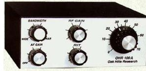
The OHR100A is currently listed on their website, and it is a single band CW transceiver kit with a RRP of USD\$179.95. Powered by 12-13.8V its current drain is nominated as
