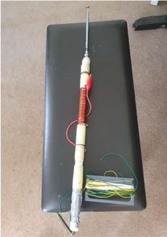
This is my Mwhip type antenna. Note the untidy coils, hand wound obviously and taped into place. There are several coils here beneath the tape as I was adding and subtracting Henries, but found the answer eventually. There are in effect now two coils, one for 20m and one more for 40m.
